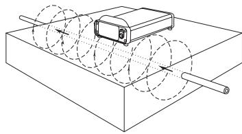
**Note:** Induction cannot be used to apply a signal to a line below reinforced concrete. the transmitter signal may be detected directly and not from the target line, so do not attempt depth measurements when closer than 15 paces from the transmitter. to check, point the receiver directly at the transmitter. if the receiver signal strength increases, either reduce the transmitter power or increase the distance from the transmitter.
