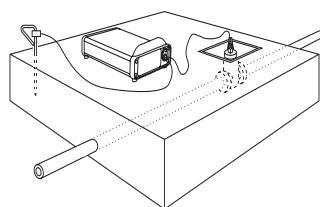
Clip the ground cable to an independent grounding point a few paces away and preferably at right angles to the probable route of the target line. Do not attach ground to water pipe or buried line which could carry the signal.
