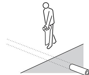
When directly over the conductor and with the sensitivity level set for a narrow response, rotate the RD2000 on its axis until the signal minimum is found. The blade is now in line with the conductor.
