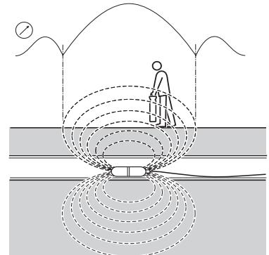
It is a good idea to locate the ghost signals as finding them positively confirms the position of the main peak. To loose the ghost signals reduce the sensitivity of the Receiver a little, leaving only the main peak signal detectable.
