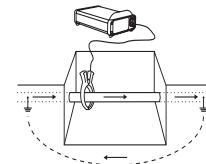
**WARNING!** to avoid the risk of electric shock, the signal clamp must be connected to the transmitter before being placed around the pipe or cable.
