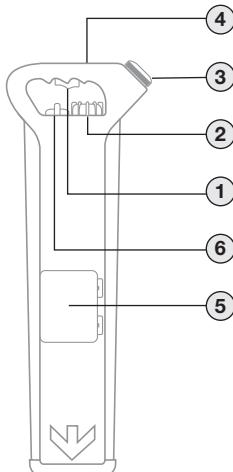
Keep the blade of the RD2000 vertical and move slowly backwards and forwards over the conductor, reducing the sensitivity for a narrower response. With the RD2000 use the meter deflection to aid pinpointing. Maximum meter deflection and audible volume from the speaker will indicate the position of the conductor
