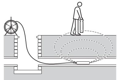
Adjust the sensitivity of the Receiver to give a bar graph reading between 60-80%.
